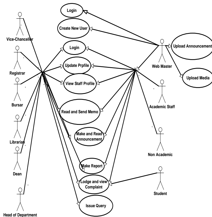
Fig. 3: Use Case diagram of the Enterprise Resource Planning Information Coordination Portal (Oyerinde I. M, 2013)
