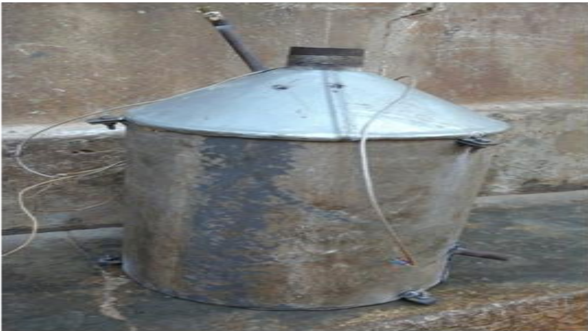
Fig. 8 Complete boiler set-up
