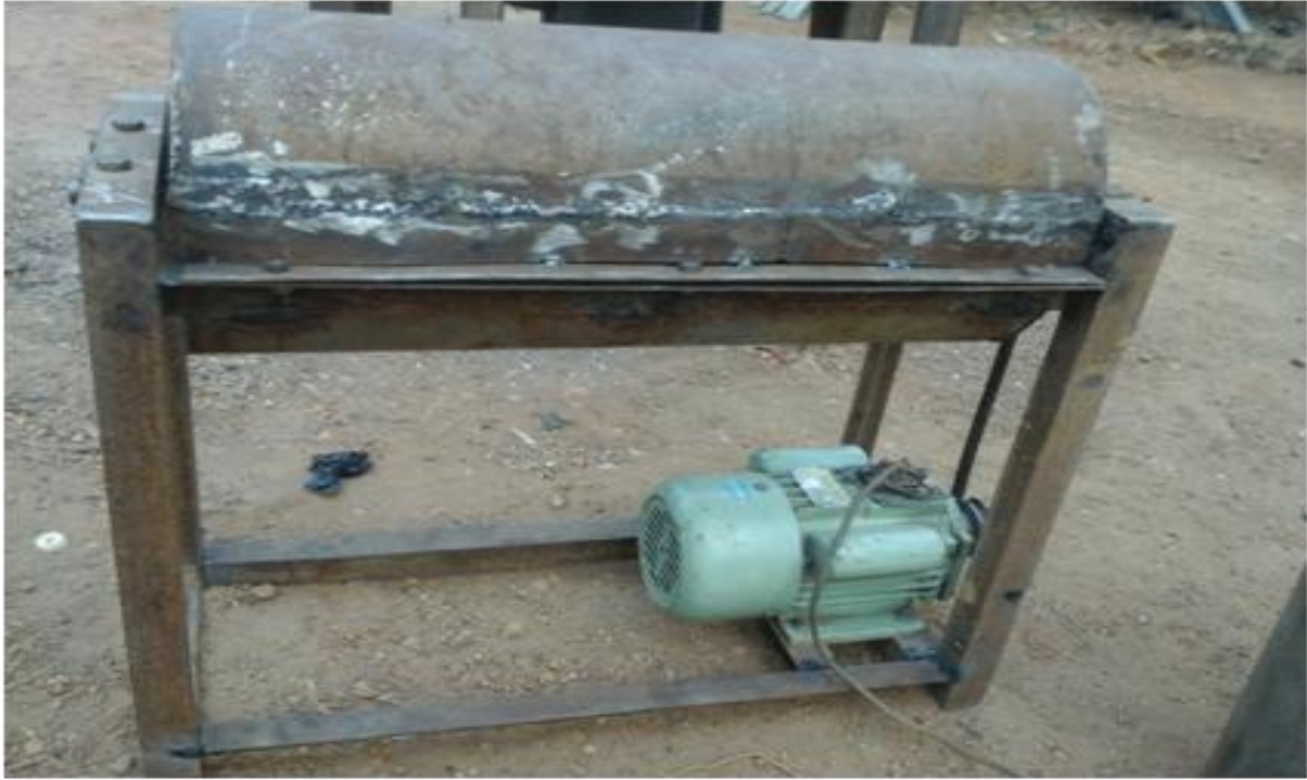
Fig. 7 Complete de-huller set-up
