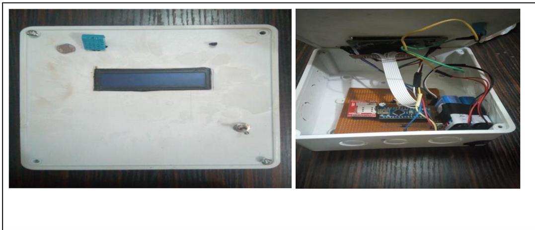
Figure 5: Implementation of the WIFI Weather monitoring system
