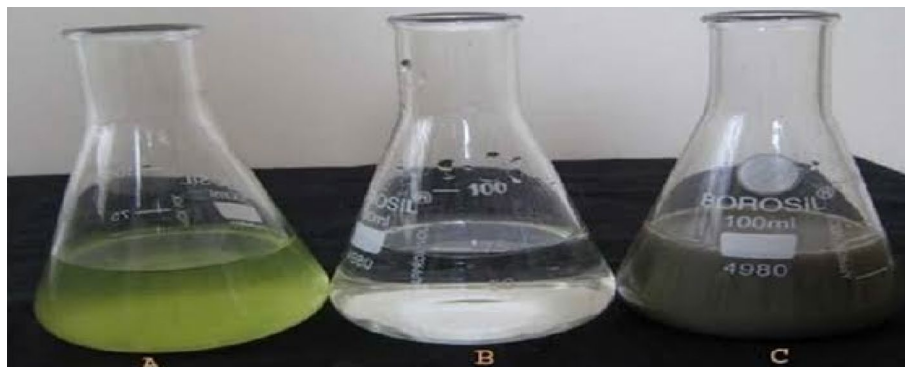
Fig. 1 Visual observation of the biosynthesis of Silver Nitrate to Silver nanoparticle (Visual inspection of colour change). A Leaves extract, B Silver Nitrate Solution, C Synthesized leaf extract
